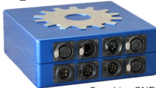
Overdrive ONE Solves position of the camera, Based on encoder data
