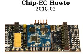
Figure 1. The Chip-EC carrier board ( with no mezzanine)
